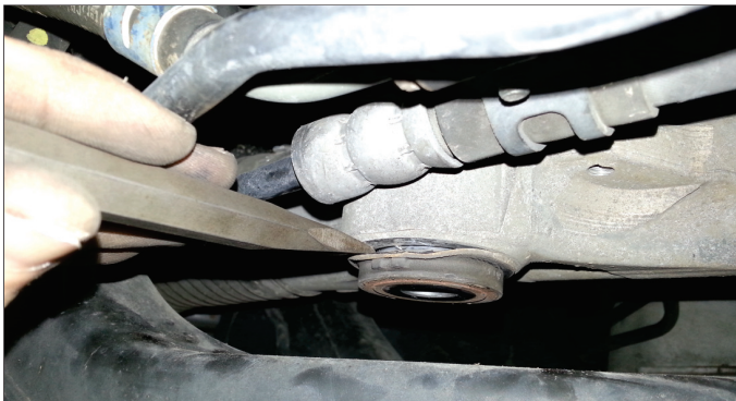
Passenger side: The rack will move toward the passenger side and forward just enough to remove the bushing. Use a Tie-Down strap to hold rack in place while removing bushing.
